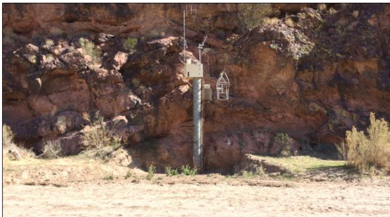
Figure 9 - USGS Continuous Stream Gage on the Hassayampa River near Morristown
